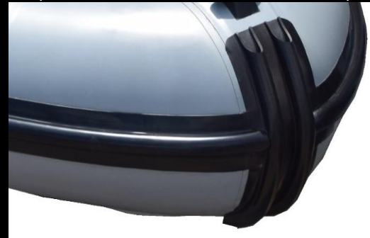
External moulded grab handles x 4 (Positioned at bow and rear of tubes)
