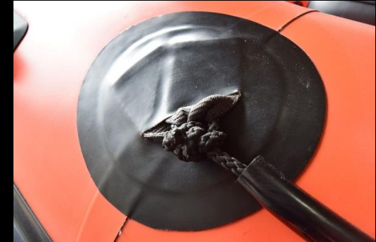
External Life lines mounted on 'D' ring safety line holders
