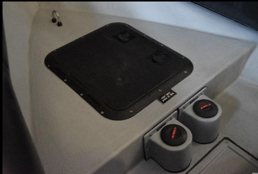
Polycarbon raised bow storage locker with two handled access hatch
