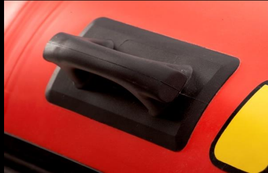
External moulded grab handles x 4 (Positioned at bow and rear of tubes)
