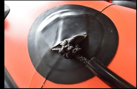
External Life lines mounted on safety line holders
