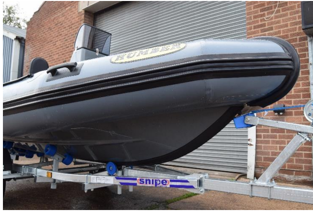
Keelguard bow protection, positionef from underside U bolt 1.5m length
