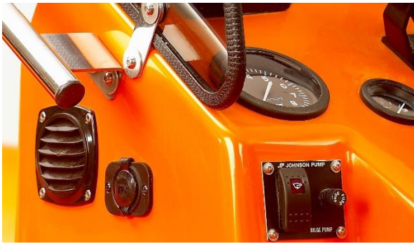
12 volt power socket with plug or twin USB socket
