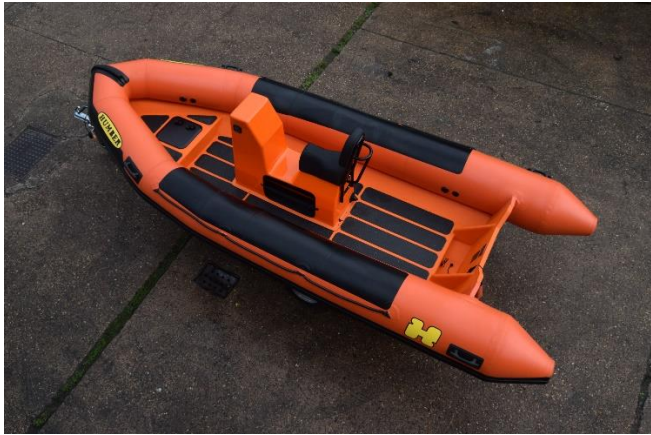
Matting, treadmaster anti-slip diamon design Pattern varies dependant on deck layout and requirements
