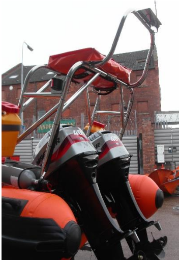
Self-Righting frame (Aluminium) with inflation bag, cylinder, valise & fitting head
