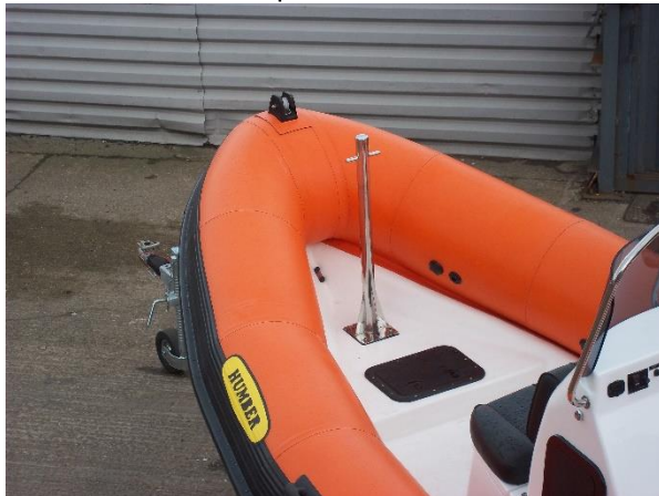
Sampson post with underside bracing Available in stainless steel or black semi-gloss aluminium
