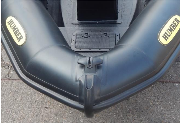
Bow jame cleat, vertical D strake & internal U bolt
